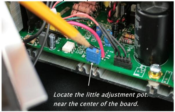
Next you will be adjusting the voltage. Connect your voltmeter to the output. Make sure the Jumper for 16 volts is in.
